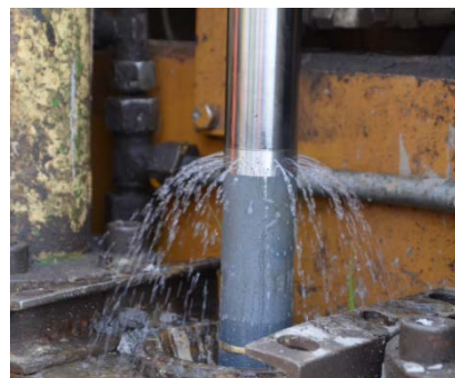
Figure 8. HPT water Injection Ports above Electrical Conductivity Sensor and standard piezocone. Photograph courtesy of Fugro
