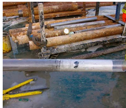
Figure 10. Geobor S Core Sample in Boulder Clay showing cored bedrock beneath clay. Photograph courtesy of Fugro.
