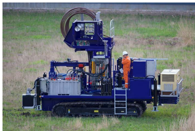
Figure 7. Deep Drive Continuous Coil CPT Rig. Photograph courtesy of Fugro
