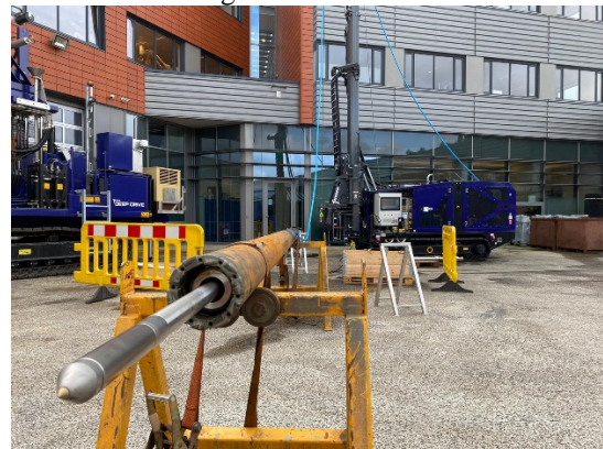
Figure 5. The Deep Line wireline CPT rig. Photograph courtesy of Fugro.
