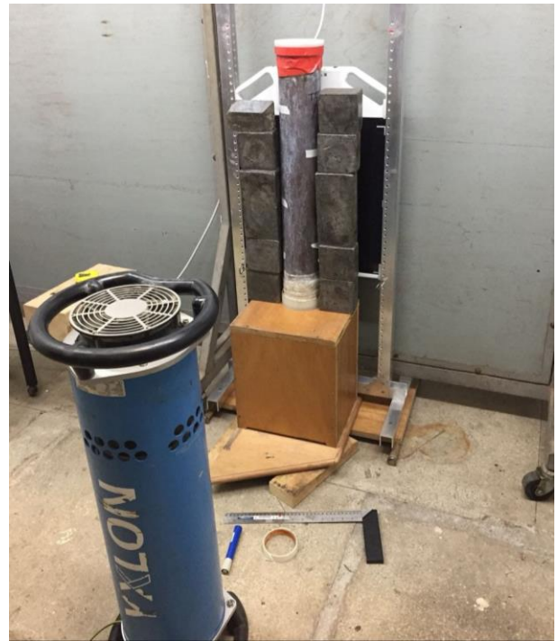
Figure 4. Positioning of radiographic equipment.
