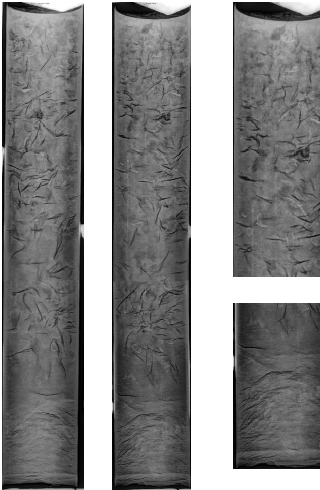
Figure 10. Radiographic images of the second sample, obtained with negative film detector. a) sample positioned at 0°; b) sample rotated at 90°; c) magnification in the upper part of the sample rotated at 90°; d) magnification at the bottom of the sample rotated at 90°.
