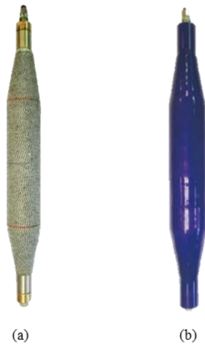
Figure 2. Photo of the probe inflated to its maximum outer diameter. (a) only the restraining sheath; (b) polyurethane sheath
