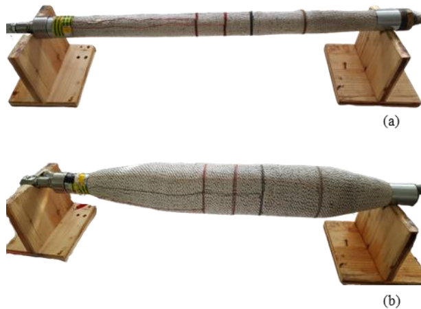
Figure 8. Probe prototype equipped with four inductance sensors. (a) deflated and (b) inflated
