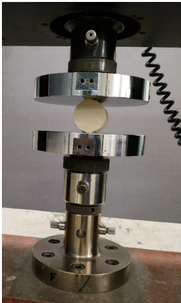
Figure 1: Brazilian test conducted to make a fracture in the sample
