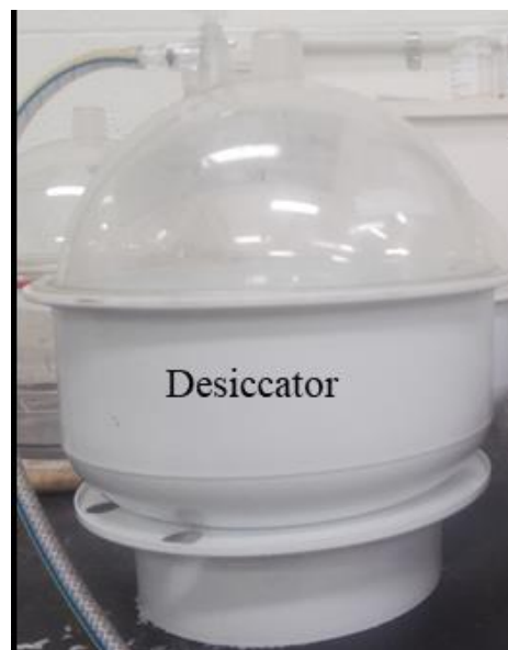
Figure 3: Desiccator used to saturate the siltstone sample
