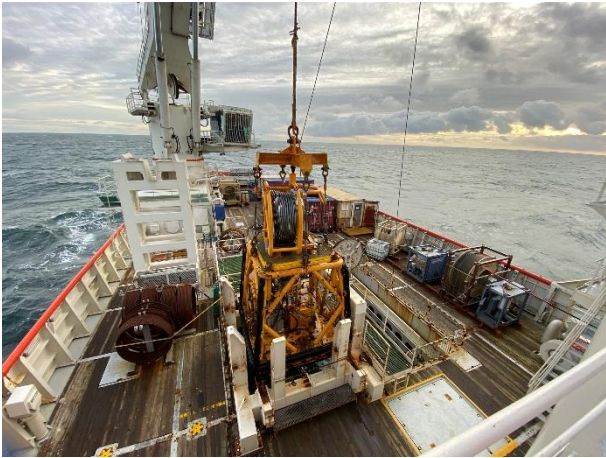
Figure 2. Offshore CPT system with coiled push rod for about 50 m penetration (courtesy Fugro)
